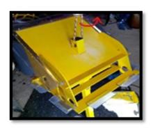
For a two piece unit, the top slope can slide off the post. The slope will have a rope (a), the post has an eye hole (b). Sometimes these will have to be removed separately.
