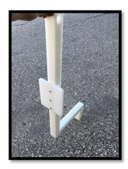
We have several variations of "spacers" used to keep shields propped in place for double catch basins. Reinstall these as you find
